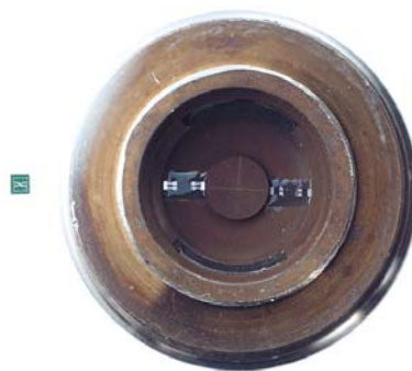
Figure 2-8: Integrated Silicon Diaphragm v Bonded Strain Gauge Design
