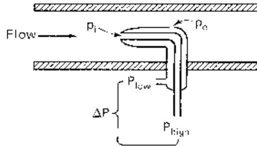
Figure 5-6: Pitot-Static Probe
