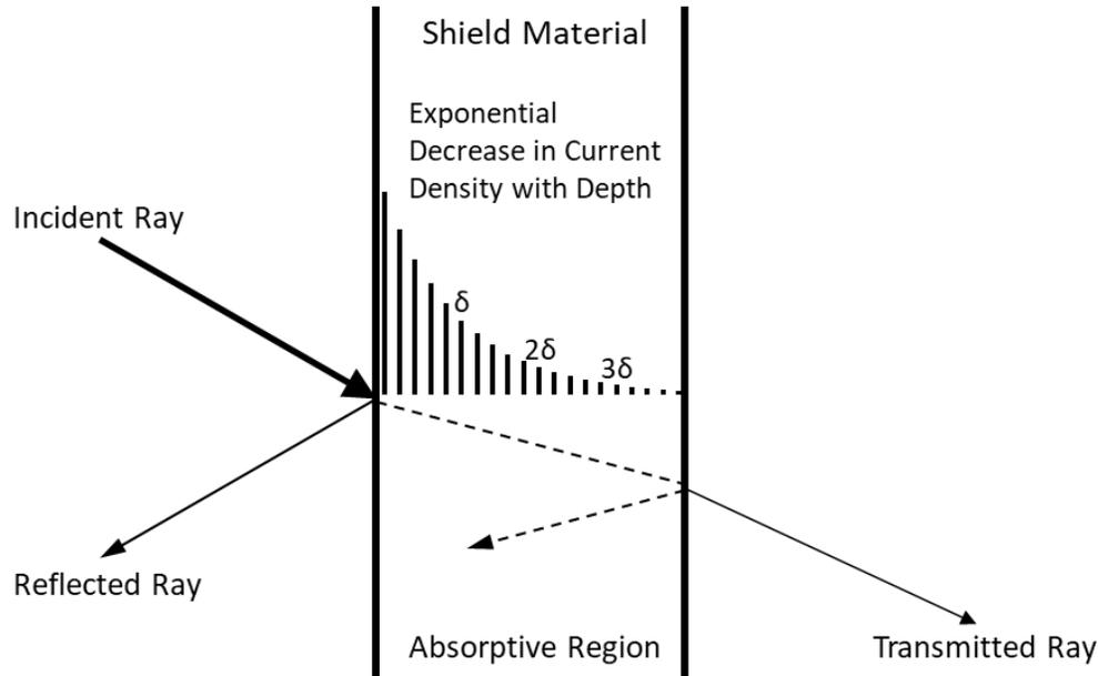
Figure 3: Reflective and Absorptive Energy Loss with Conductive Shielding
