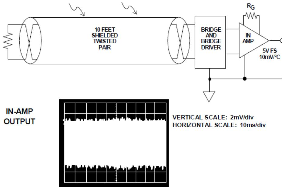
Figure 4: Ungrounded Shielded Cables Act as Antennas
