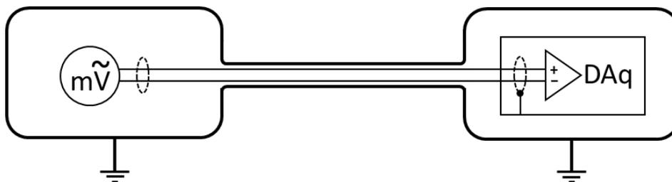
Figure 1: Low-Level Dynamic Signal Shielding with Faraday Enclosure
