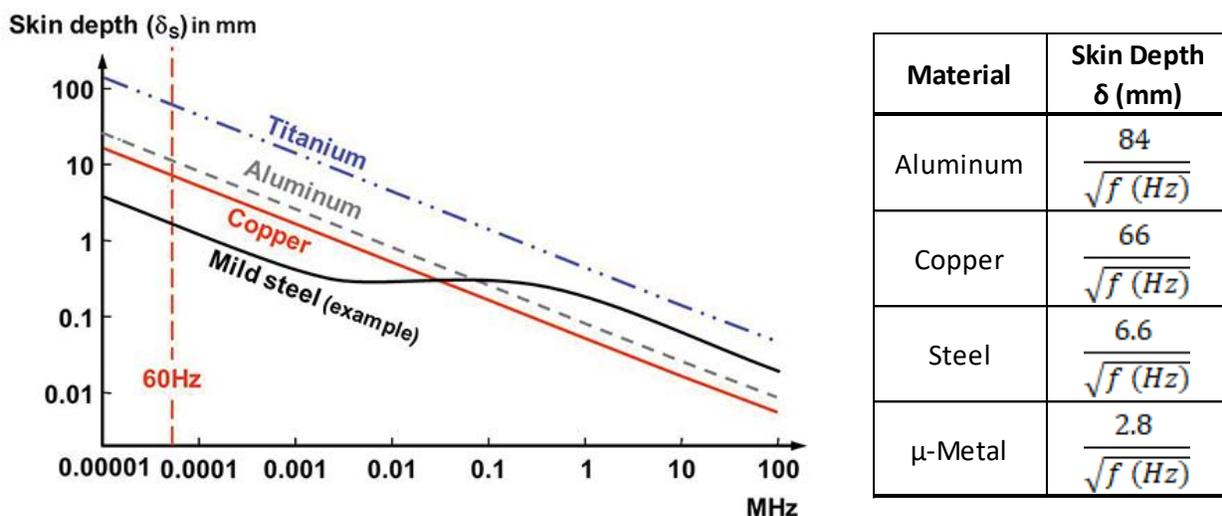
Figure 2: Skin Depth vs. Frequency for Common Enclosure Materials
