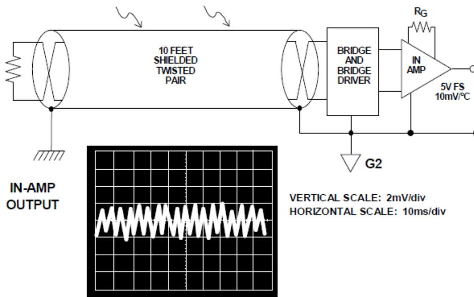
Figure 5: Grounding Both Ends of a Shield Produces Low Frequency Ground Loops
