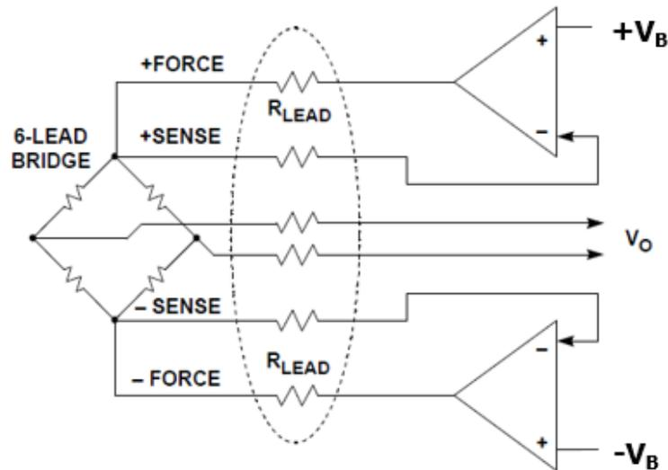
Figure 2: Balanced Bipolar 4-wire Kelvin Voltage Excitation
