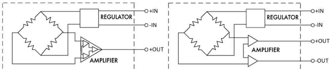
Figure 1a: 3-Wire Amplified Voltage Output
