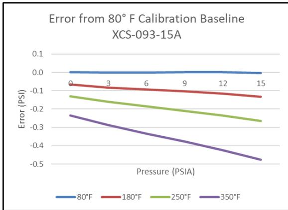
Figure 5a: Typical Thermal Error at Temperature
