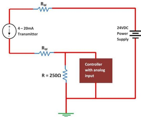
Figure 2: Simple 4 to 20 mA Current Loop Schematic
