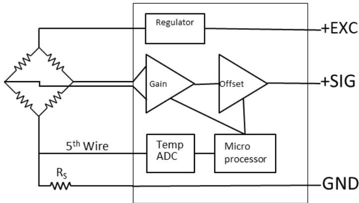
Figure 6: SOI Pressure Sensor Interface to ASIC
