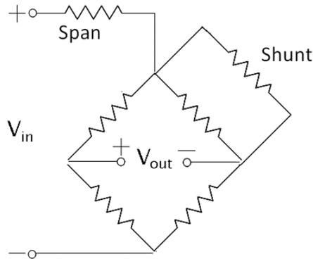
Figure 3: Simple Thermal Compensation of SOI Pressure Sensor
