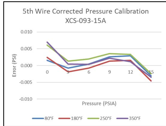
5b: Corrected Thermal Error Using 5<sup>th</sup> Wire
