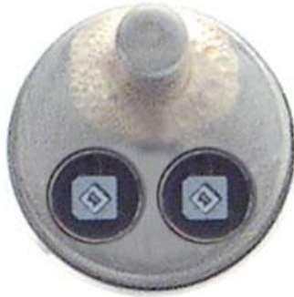
Figure 6 - Silicon Sensing Die with Wheatstone Bridge
