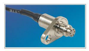
The KZSM/T-400 is a miniature flange mount pressure transducer/platinum RTD combination. The pressure transducer utilizes a patented silicon on silicon design. The integrated platinum RTD is used to sense media temperature. The pressure and temperature devices are designed to operate independently. All wetted parts of the transducer are compatible with most automotive fluids.
