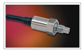
The MAKS-6(X) is one of the newest generation of Kulite's smallest miniature amplified transducers currently available. The sensing sub-assembly is protected from mechanical damage by a protective screen, which has been shown to have minimal influence on the frequency response of the sensor.
