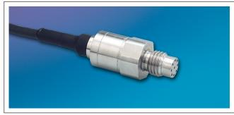
piezoresistive sensing element via thin intervening film of non-compressible silicone oil. This sensing sub-assembly is protected from mechanical damage by a protective screen, which has been shown to have minimal influence of the frequency response of the sensor.
