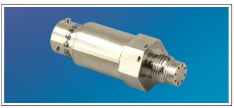
ETL-DC-375(M) CO Series transducers are miniature, threaded instruments. The sensing sub-assembly is protected from mechanical damage by a solid screen which has been shown to have minimal influence on the frequency response of the sensor. The ETL Series uses Kulite's Patented Leadless Technology.
