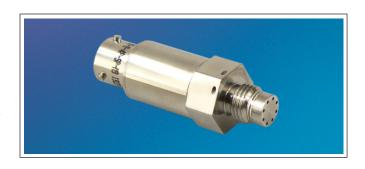
Incorporation of a Kulite proprietary electronics module within the main body of this product allows for operation from an unregulated power supply ranging from 12  $\pm$  4VDC or 28  $\pm$  4VDC with reverse polarity protection available upon request. Part performance not guaranteed if used in water.
