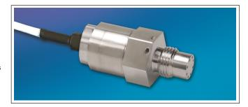
ETL-200-375 Series transmitters employ the same approach to transducer construction as the standard ETL-375 Series. The ETL Series uses Kulite's Patented Leadless Technology. The Kulite proprietary electronics module in this product line, however, provides a current output signal (4 to 20 mA). These instruments are an excellent choice for applications requiring the current output signal but in which space and/or weight are at a premium.
