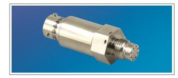
ETL-200-375(M) CO Series transmitters employ the same approach to transducer construction as the standard ETL-375(M) CO Series. The ETL Series uses Kulite's Patented Leadless Technology. The Kulite proprietary electronics module in this product line, however, provides a current output signal (4 to 20 mA). These instruments are an excellent choice for applications requiring the current output signal but in which space and/or weight are at a premium.
