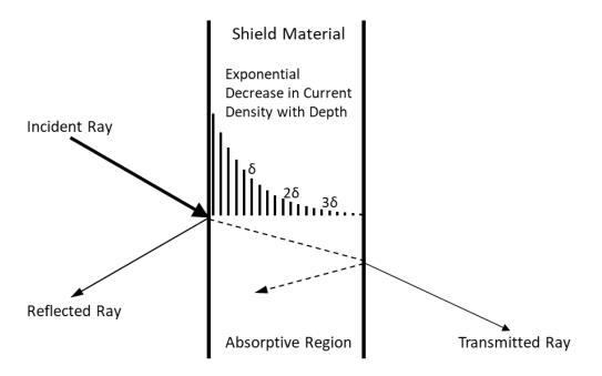
Figure 3: Reflective and Absorptive Energy Loss with Conductive Shielding
