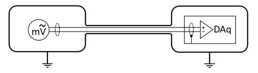
Figure 1: Low-Level Dynamic Signal Shielding with Faraday Enclosure
