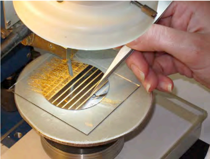
Strain Gage Lead Attachment (In Process)
