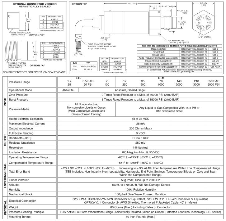
Note: Custom pressure ranges, accuracies and mechanical configurations available. Dimensions are in inches. Dimensions in parenthesis are in millimeters. All dimensions nominal. (O) Continuous development and refinement of our products may result in specification changes without notice. Copyright © 2014 Kulite Semiconductor Products, Inc. All Rights Reserved.
