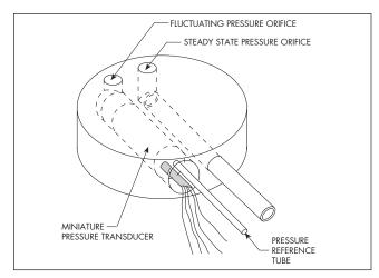
These probes are particularly suitable for rake fabrication. Two techniques which have been very successfully employed are shown below:
