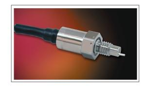
The MAKS-6T(X) is one of the newest generation of Kulite's smallest miniature amplified transducers currently available. The sensing sub-assembly is protected from mechanical damage by a protective screen, which has been shown to have minimal influence on the frequency response of the sensor. Incorporation of Kulite proprietary high temperature 392°F (200°C) electronics within the main body allows for operation from an unregulated power supply of 8 to 16VDC.
