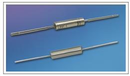
measurements and dynamic pressure measurements in which the reference tube is also exposed the measurand. The compact LPF design enables the device to be easily attached via soft, elastic tubing to the reference tube of a differential pressure transducer. In-situ static pressure calibration can easily be conducted through the LPF. The LPF can quickly be removed to reuse the transducer for a different test application.
