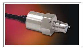
The ETL/T-HT-375 is a miniature threaded pressure transducer/ platinum RTD combination. The pressure transducer utilizes a patented silicon on silicon design. The platinum RTD protrudes beside the diaphragm to sense media temperature. The pressure and temperature devices are designed to operate independently. All wetted parts of the transducer are compatible with most industrial and automotive fluids.
