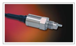
The ETL/T-312 is a miniature threaded pressure transducer/platinum RTD combination. The pressure transducer utilizes a patented silicon on silicon design. The platinum RTD protrudes beside the diaphragm to sense media temperature. The pressure and temperature devices are designed to operate independently. All wetted parts of the transducer are compatible with most automotive fluids.
