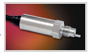
The EPTS-312 is a miniature threaded pressure transducer/platinum RTD combination. The pressure transducer utilizes a patented silicon on silicon design.
